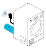
These dryers use electric resistance heaters to dry your clothes and require a vent to the outside to get rid of warm, moist air.
