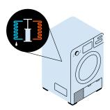
These dryers use a heat pump refrigeration cycle that moves heat. In this case they move heat into the air entering the dryer drum and pull heat from the air that exits the dryer drum to condense out the water into a drain or pan. That same air is then reheated before returning to the dryer drum. Think of it as a very efficient way of moving water from your clothes to the drain.
