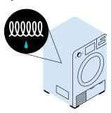
Condensing dryers use electric resistance heaters for drying, but instead of a vent to the outside they have a separate cooling element that acts like a dehumidifier to condense the water from the moist air, collecting it in a pan or sending it down a drain. They are more efficient than electric dryers and are handy when venting to the outside is not an option.
