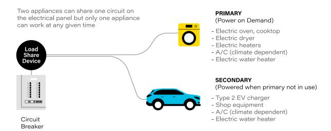
Load share device with primary and secondary loads allow two appliances to share one circuit and one breaker on the electrical panel. Only one of the appliances can be in use at one time. The primary load has the power by default and the secondary load can only draw power when the primary load is off. For example, a stove may be
