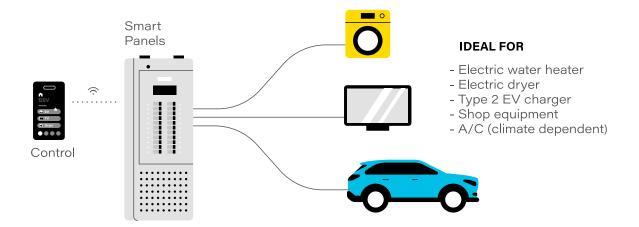
Smart electrical panels monitor power use in real time and use software to allow for load management across multiple circuits. They generally replace the existing panel. Where permitted, homeowners can program the panel to fit more electrical loads on the panel by prioritizing some appliances over others. Smart panels also help optimize when energy is used to save money in
