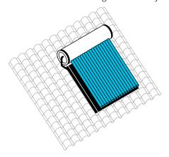
be very simple and reliant on passive movement of the heated water, or they may be more complex with fancy collectors and pumps to move water. In colder climates, fluids circulate between the collector and the water tank where the heat is transferred to the water in the tank using an exchanger. Because the sun doesn't always shine, these systems require an integrated backup water heater.
